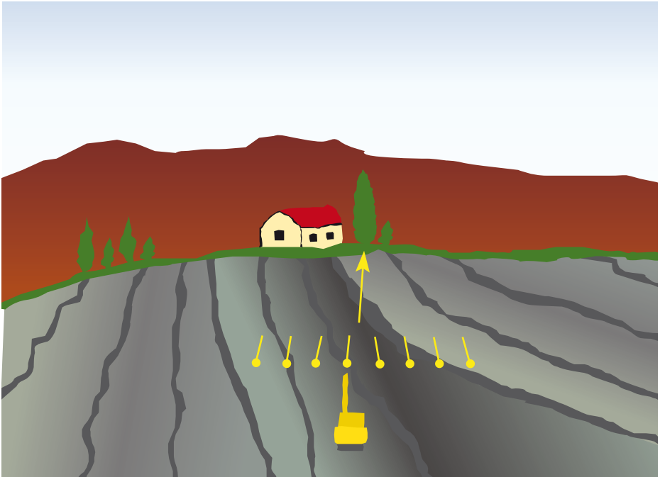
Conventional positioning. The drill rig and feed are aligned with a landmark in the distance. Note that the resulting holes are not parallel.
